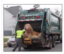
Leaf collection is a Mobile Work Zone. Establish traffic control according to the MUTCD. At a minimum, high intensity amber warning lights must be visible to motorists approaching from either direction.
